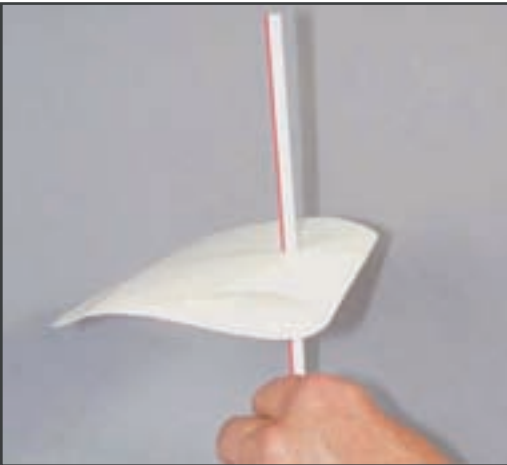
Scissors or a hobby knife can be used to cut a hole in the upper and lower curved surface (called the camber)
