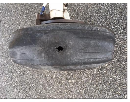
In one mishap, a pilot and another member were on a proficiency sortie. The sortie proceeded uneventfully and the pilot was going to end the mission with a practice shortfield approach and landing. As both members relate, the approach and landing were fine, up until "the pilot immediately applied strong braking pressure" which resulted in a skid causing one flat-spotted tire and one tire worn all the way through until it went flat.
