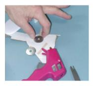
Step 9 - A bead of hot glue is run down the front of the fuselage as shown. Using the lead photograph on this activity, and the illustration, mount the landing gear strut into the correct position.
