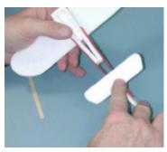
Step 8 – To make the landing gear, you must first mount the fender washers onto the wooden coffee stirring sticks. Cut the stick down to size by using the template as your guide. Then put a glob of hot glue on one tip and press a washer down into the glue. Cut a piece of wood and press this into the glue that oozes through the center of the fender washer. This will hold the "wheel" in place. Make two!
