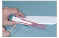
Step 4 – Glue the rudder to the ends of the four fuselage stirring sticks.
