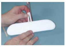
Step 7 - The horizontal stabilizer is mounted at the back near the rudder. Note that it is on the bottom of the fuselage coffee sticks. Check the illustration on how this is positioned.
