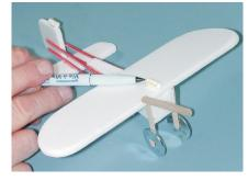
12. Finally, another short soda straw is mounted to the upper portion of the wing to make the second "carrier" for the fishing line.
