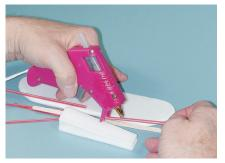
2. Run a hot glue bead along the edge of a plastic coffee stirring sticks, as shown.
