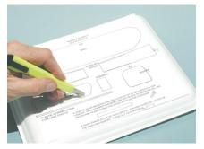
1. Tape template to bottom side of tray. Then cut out pieces with knife.
